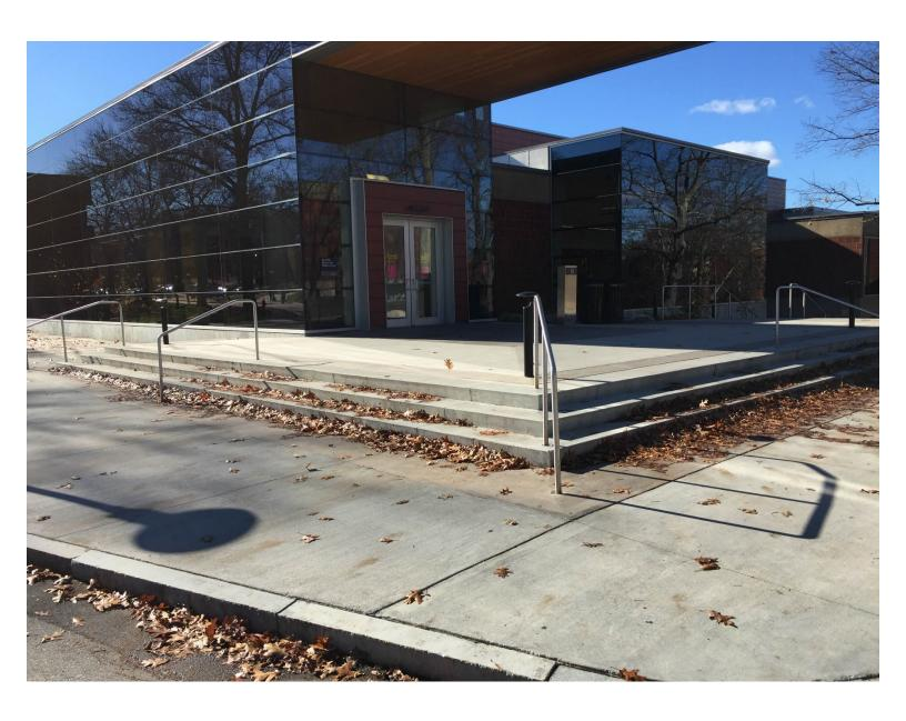
This feature contains Concrete Ramp. There are Ramps/Walkways 6 feet wide and approximately 39 | Total Area: 234 square feet. feet total length.
